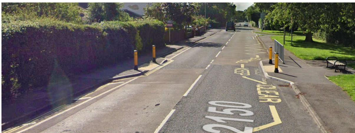
Figure 26 – Example of a road narrowing with pedestrian crossing facilities
