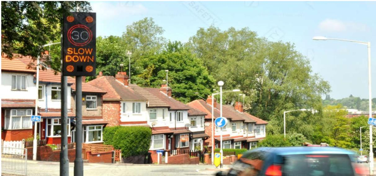
*Figure 12 – Example of basic VAS displaying speed limit*
