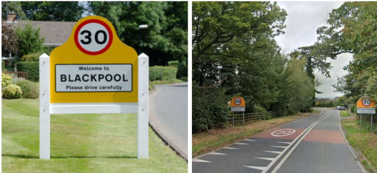
Figure 8 – Examples of speed limit gateway treatments
