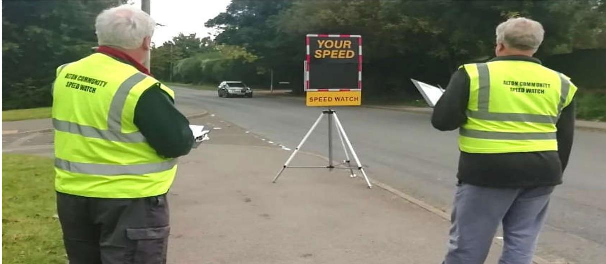
*Figure 14 – Example of mobile VAS displaying vehicle speed*
