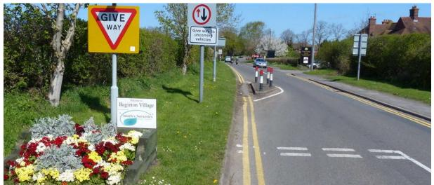
Figure 25 below provides an example of a priority give-way system in operation.
