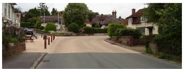
Figure 11 – Example of changing the surface colour to enhance the environment
