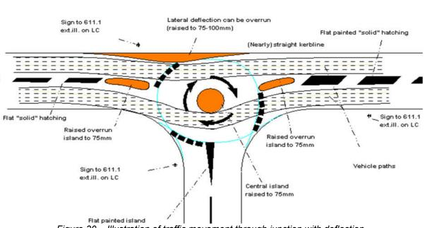
Figure 29 – Typical example of a mini roundabout
