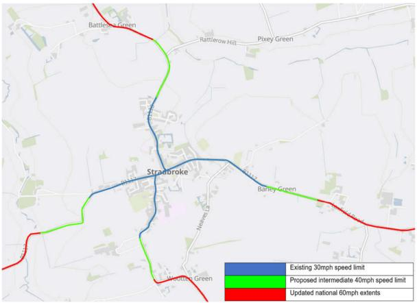
Figure 9 – Proposed intermediate 40mph speed limit on the approaches to the village
