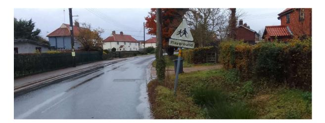
Whilst a number of the signs are in poor condition there are also locations where there is no signage, where there could be a benefit, such as advance warning signage. Positioning these signs in appropriate locations may assist in the control of speed on the approach to the centre of the village.
