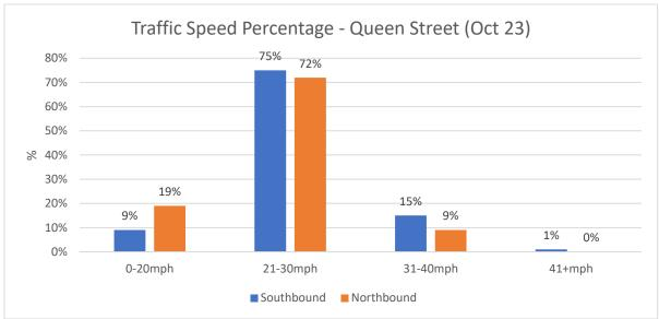
Figure 4 – Breakdown of traffic speed from ATC survey along Queen Street Oct 23
